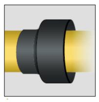
Insert the end seal on the main pipe before inserting the casing pipe otherwise the final connection of the pipeline.
